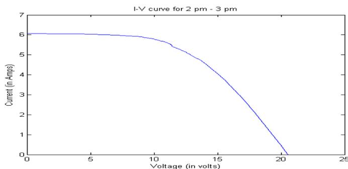
Fig. 4 V-I characteristics of a PV System
